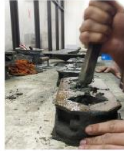
Tamping the mold
