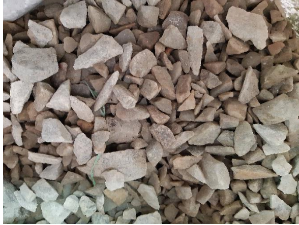
Figure 6.7: Stone chips used as coarse aggregates
