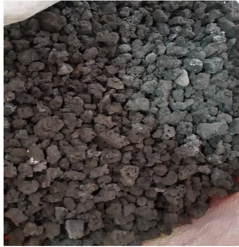
Figure 6.9: QEAF slag of size 3/4 inch downgrade used as coarse aggregate replacement
