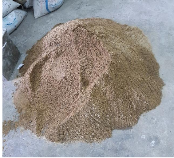
Figure 6.1: Sylhet sand as fine aggregate
