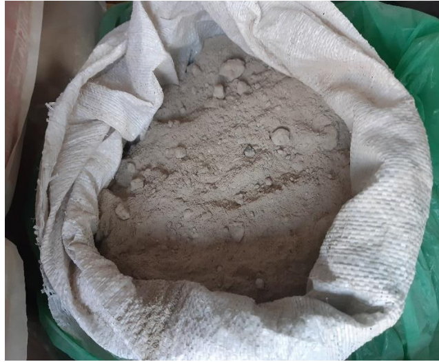
Figure 6.5: LRF slag used as fine aggregate replacement
