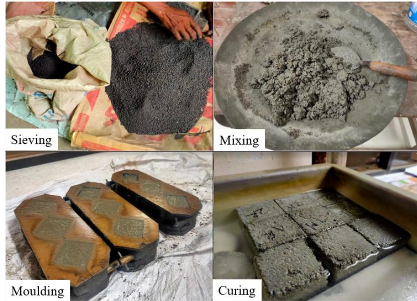
Figure 10.1: Different stages of Block Manufacturing Process.
