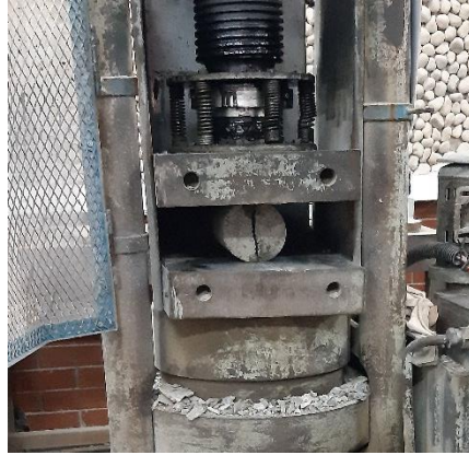
Figure 6.15: Splitting Tensile Strength Test
