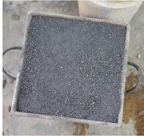
Figure 6.3: QEAF slag of size 5 mm downgrade used as fine aggregate replacement
