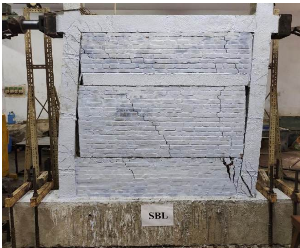
Figure H.12- SBL at complete failure.
