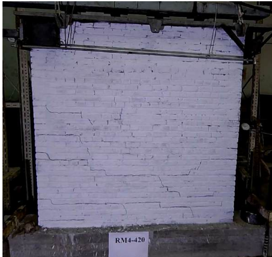
Figure 4.9- RM4-420 after the completion of cycle 7.
