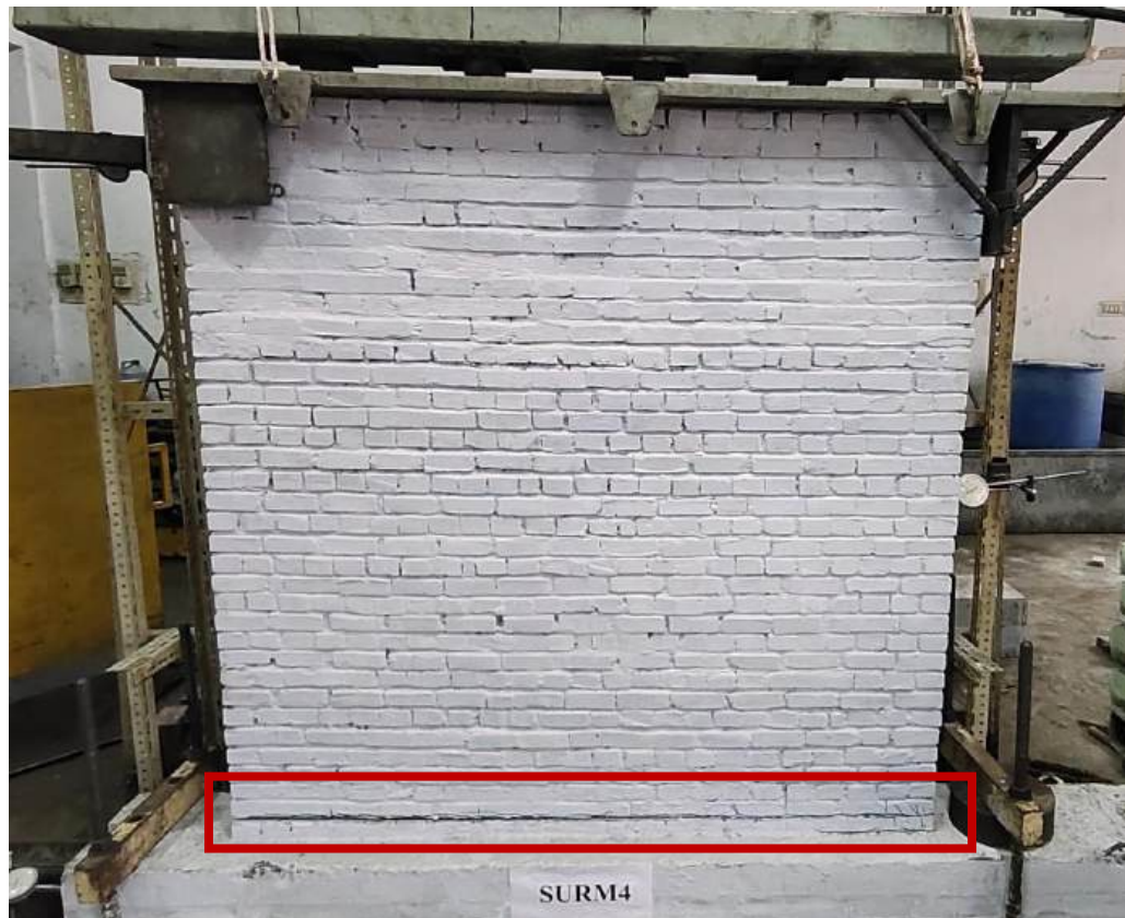
Figure 4.1- SURM4 at complete failure.
