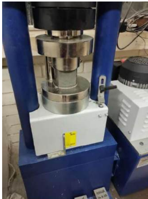
Figure D.1- Prepared mortar cubes mortar testing.
